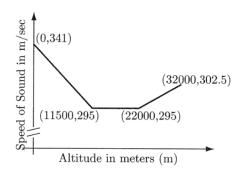
In the earth's atmosphere the speed of sound is a function of the altitude. The figure above, consisting of three line segments, shows the speed of sound, s(a), in meters per second as a function of altitude, a, in meters. The graph is not drawn to scale. What is the average speed of sound in meters per second on the interval [0,32000]?
